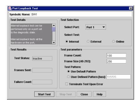
Figure 5-4. Port Loopback Test Dialog
